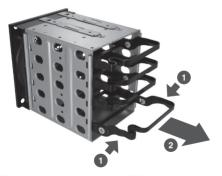
Press both side bars of HDD tray, then pull the HDD tray out from the module to begin installation.
