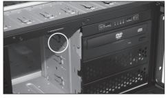
5. You can slide the ODD back in to complete the installation. Make sure the round shape button has locked with the ODD rail. You can also remove the ODD by pressing the button, then pull out.
