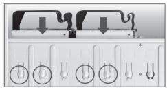
1. First press the two round shape buttons using your thumbs, then use your index finger to push the 3.5" module to remove it.
