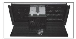
2. Pull the module out from the front panel.
