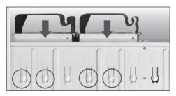
First press the two round shape buttons using your thumbs, then use your index finger to push the middle 3.5" module to remove it.
