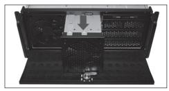
2. Pull the module out from the front panel.
